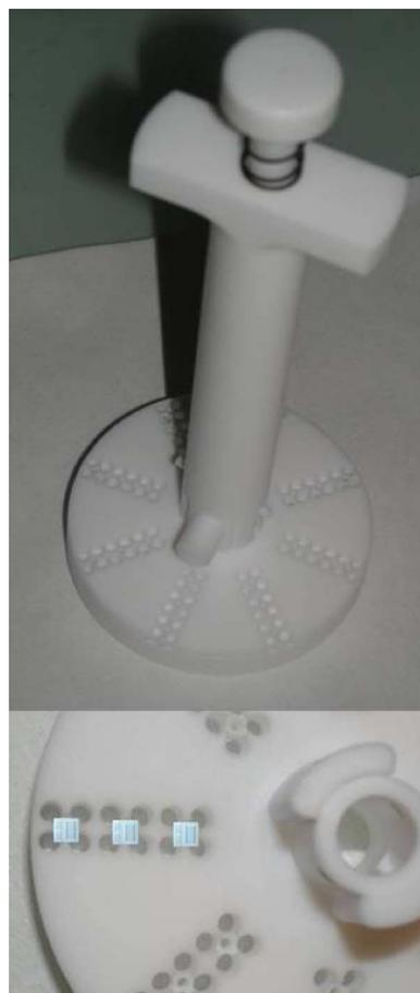
Fig. 4. Photograph of the chip holder which can be used for wet processing of twenty-four  $3\text{ mm} \times 3\text{ mm}$  die. The handle is removable so that the base with the chips can be loaded into the supercritical point dryer. The inset at the bottom of the figure shows the base of the holder (handle and chip cover plate removed) with  $3\text{ mm} \times 3\text{ mm}$  chips in the cavities.
